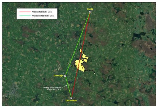
Figure 11. Example of how an existing telecoms mast could be relay the radio link between Cloonriddia and Castle.
