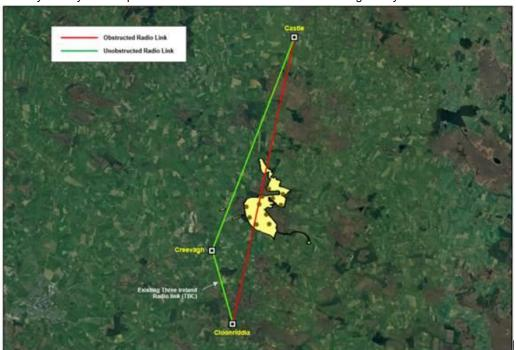
Figure 11. Example of how an existing telecoms mast could be relay the radio link between Cloonriddia and Castle.
