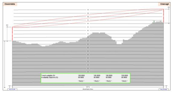
Figure 12. Path Profile - Cloonriddia to Creevagh
